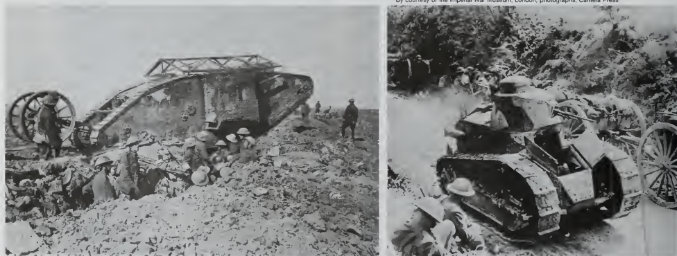
Figure 23. Tanks of World War I. (Left) British Mark I tank with antibomb roof and "tail," 1916. (Right) French Renault F.T. light tank, 1918.
